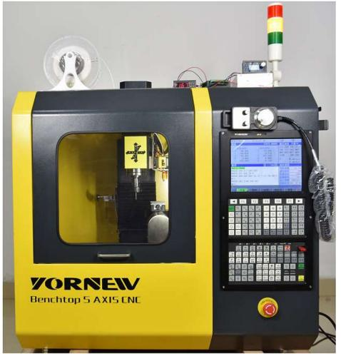
We converted a desktop 5-axis subtractive machine (YORNEW Benchtop 5 Axis CNC MX220) into a simple 5-axis hybrid machine by adding an external additive extruder parallel to the tool spindle.
